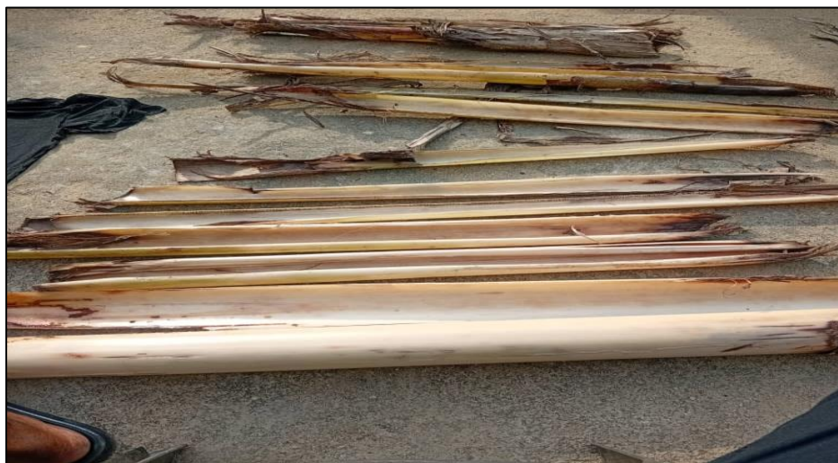
Figure 3 Extraction of Musa paradisiaca fibres
