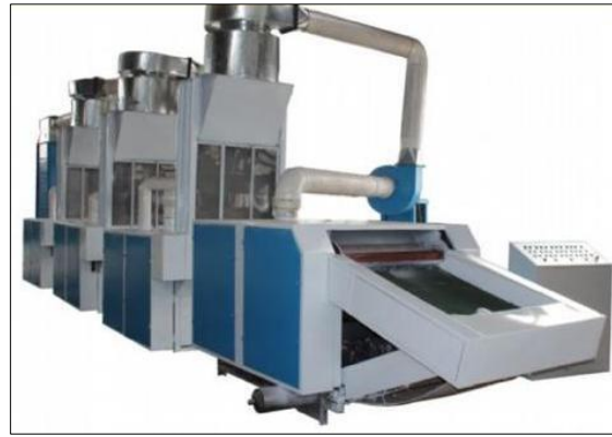
Figure 2 Waste recycling machine
