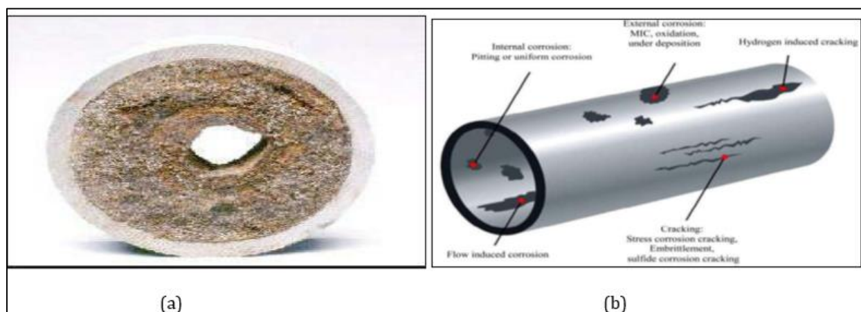
Figure 1 (a) Wax deposit in a retrieved pipeline (b). Oil pipeline corrosion
