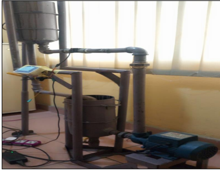
Figure 2 Complete experimental flow loop set-up
