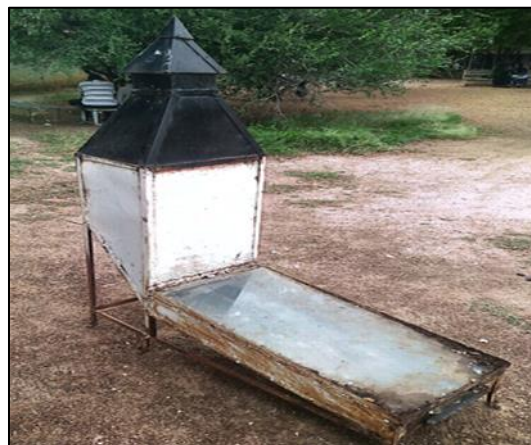
Figure 1 Natural convective solar dryer dryer Ddryer PLATE 1
