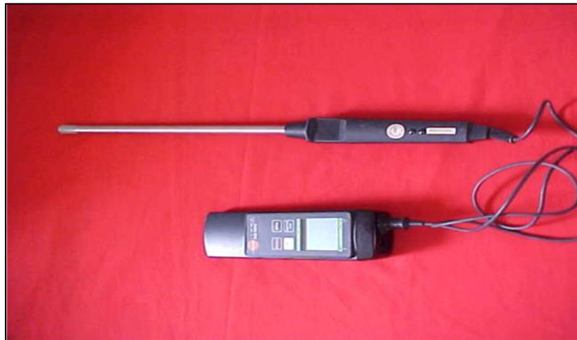
Figure 3 Digital hygrometer for measuring relative humidity (%)
