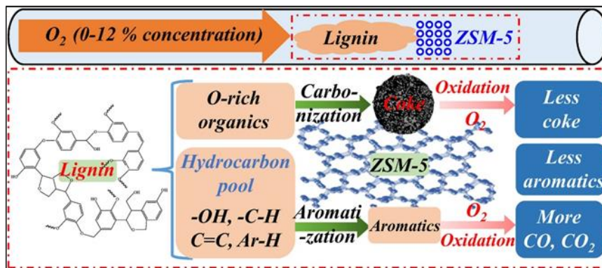
Figure 4 Reaction mechanism during the catalytic pyrolysis of lignin with ZSM-5 as catalyst in the presence of O_2 [118]
